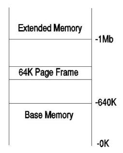
can be allocated to a program, but only one will be in the address space of the CPU at any time, as that bank is switched, or *paged*, in as required. In other words, the program code stays in the physical cells, but their electronic address is changed, either by software or circuitry.
