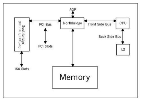
Essentially, the functionality of the chipset is combined on two main components, the North- and South- Bridge chips, which live at each end of the PCI bus. The CPU, Memory and AGP talk to the Northbridge and the Southbridge handles all the I/O, including the ISA bus. NVidia calls them the IGP and MCP, respectively, standing for Integrated Graphics Processor and Media and Communication Processor (their chipset also uses AMD's Hypertransport technology, which is mentioned below).
