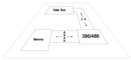
In view of the above, you can see that processor speed alone is no guide to performance, and in some cases may even be irrelevant. A slow hard disk (on the data bus), for instance, will always make any processor wait for its data and waste cycles that could be used for serious work. In fact, as far as NetWare is concerned, a 486/33 is only noticeably better than a 386 when network loading is heavy.
