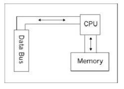
The Central Processor does all the thinking, and is told what to do by instructions contained in memory, so there is a direct two-way bus connection between them—the *bus width* (multiplied by its frequency and number of times data is transferred per clock cycle) determines how much data can be read or written in one go.
